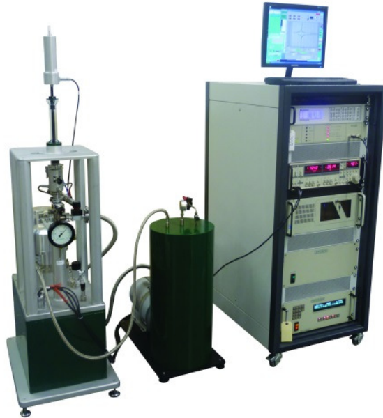
Figure 1: MiniCFMS shown with VSM option
