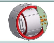
One solenoid and two split pairs or three split pairs allowing rotation of the field in any orientation and sample axes along the three axes.
