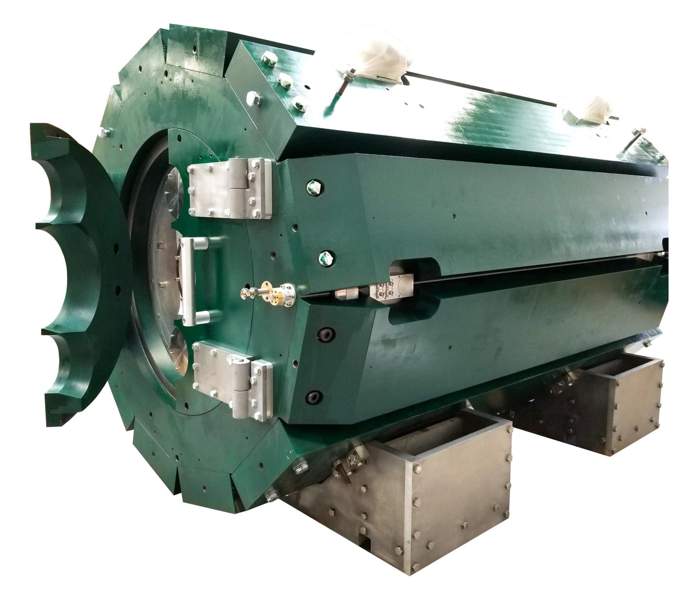
The magnet produces a homogeneous field profile with a maximum 2.6 T over a large cylindrical volume of Ø70 cm × 200 cm. The field is generated using four individually controllable solenoids. Subtle changes in the field profile are possible by varying the individual coil currents.
