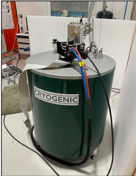
System consist of 9.4T NB magnet Techmag Redstone console and Phoenix 4 mm probe
